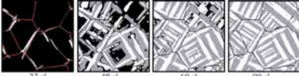
Fig.3 Evolution of tetragonal phase without PA in polycrystalline material containing 7 parent grains.
